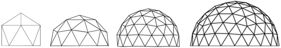
Fig. 5.2 - Dome geometry and frequencies
